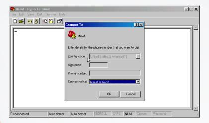
Step 5: Configure the port parameter settings. Bits per second: "115200", Data bits: "8", Parity: "None", Stop bits: "1", Flow control: "None". Click OK
